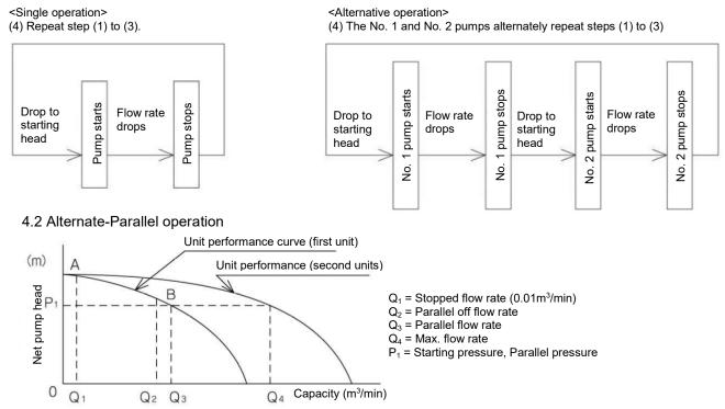
(1) When water is used while the pump is stopped and the pressure drop to P<sub>1</sub>, the pressure sensor detects the pressure, and pump starts.
