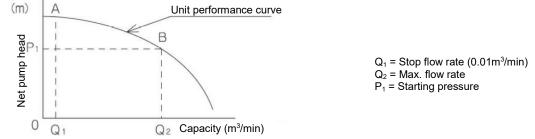
(1) When water is used while the pump is stopped and the pressure drop to P<sub>1</sub>, the pressure sensor detects the pressure, and pump starts.
