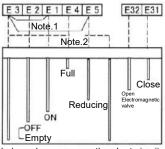
(Note 1) In the case of using the electrode bar, please remove the short-circuit wire between E3 and E1.
