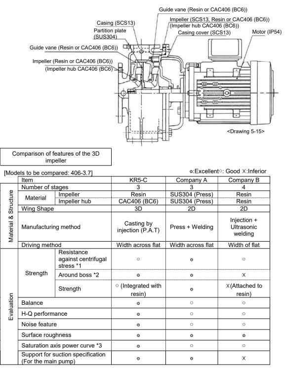
\*1: The centrifugal stress on the impeller is proportional to the impeller's specific gravity.
