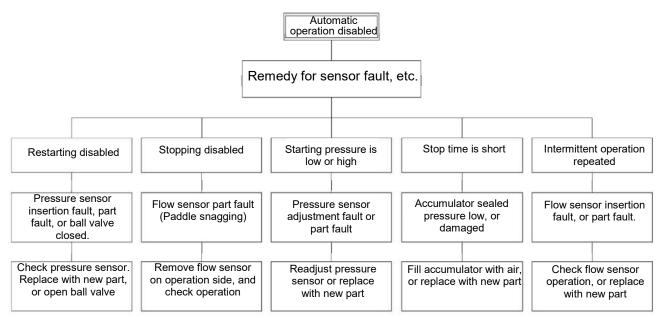
\*1. The flow sensor is designed so that the pump will stop when the sensor is disconnected from the connector.
