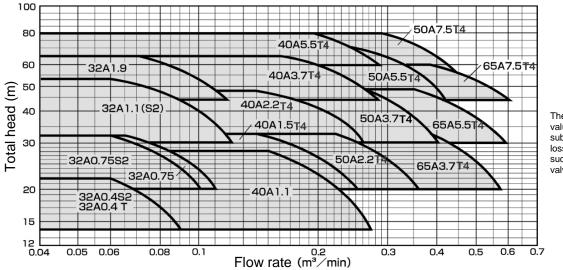
The specification values are after subtracting the losses in the unit such as the check valve etc.
