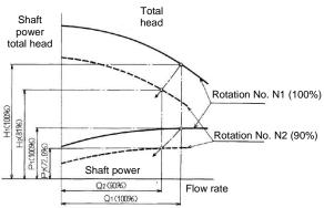
[Drawing 3-1] Relationship between the pump's characteristics and rotation speed
