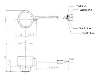
Specification 1 Rated voltage: DC12V 2 Output form: DC1-5V 3 Maximum working pressure: 0.97MPa (9.9kgf/cm<sup>2</sup>) 4 Pressure change: Within  $-{}^{0}_{3}\%$ 5 Noise resistance: 1500V×1  $\mu$  sec
