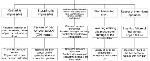
\*1. If removing each sensor from the connector, the pump stops or operates slowly.
