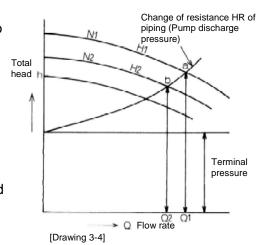
is that the variable range of terminal pressure is small.
