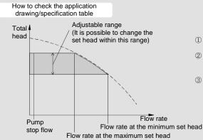
The total head is shown as the value after subtracting the losses of check valve (shock-less valve) etc. from the pump performance.
