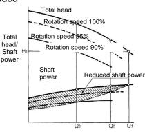
[Drawing 3-2] Comparison of shaft power at the time of rotation speed change
