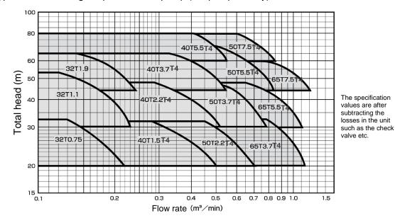
KF2-T Type selection charge, Operation of 3 pump (3/3 pumps rotary)
