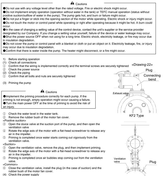
$\bigcirc$  Confirm that the voltage is within 200V $\pm$ 10% by turning the power ON, turn the earth leakage breaker in the control panel ON, operate the display panel on control board, and then display the power voltage.
