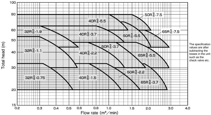
Operation of 6 pump: 6/6 pump rotary
