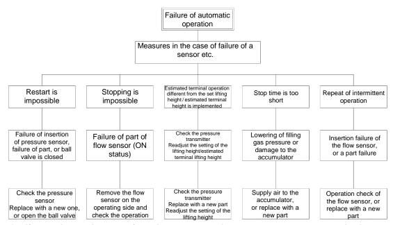
\*1. If removing each sensor from the connector, the pump stops or operates slowly.
