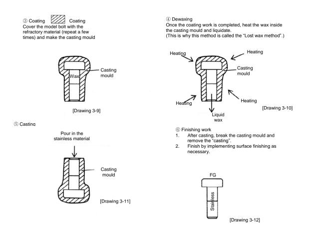
(3) Comparison between the lost wax method and sand mold casting
