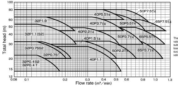
The specification values are after subtracting the losses in the unit such as the check valve etc.
