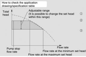
The total head is shown as the value after subtracting the losses of the check valve (shock-less valve) etc. from the pump's performance.
