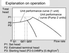
■ Alternate operation ① If water is used while the pump is not operating and the pressure decreases to P3, the pump starts
