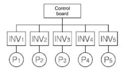
• In the case of the drawing at left, if a failure of the control board occurs, all the pumps become inoperable, causing a water supply failure.
