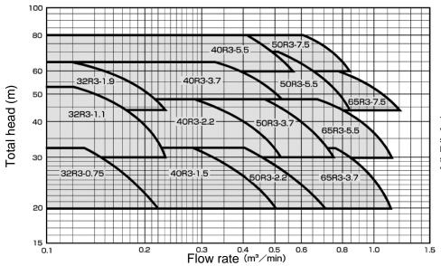
The specification values are after subtracting the losses in the unit such as the check valve etc.
