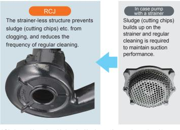
\* Dischargeable cutting chip length: Aluminum: 40 mm or less; other: 15 mm or less
